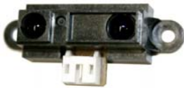
Fig. 4. GP2D120 Infrared sensor, left-hand light emitter, right-hand light detector
