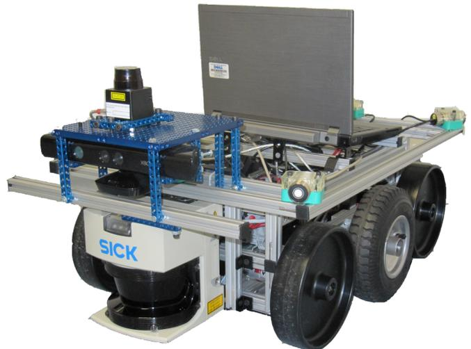
Figure 1. Our robotic platform prepared with the three sensor systems – Hokuyo URG-04LX-UG01, Microsoft Kinect, SICK LMS200 – for navigation tasks
