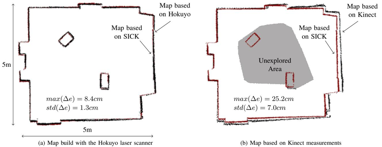
Figure 3. Comparison of occupancy grids generated with different sensors. The results of a SICK LMS200 were added as a reference with red dots.
