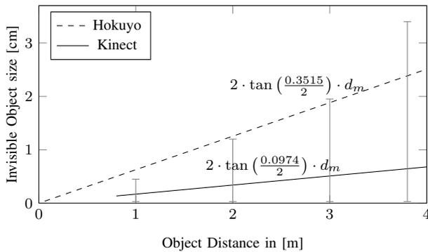
Figure 2. Theoretical size of invisible objects related to the angular resolution for different obstacle distances  $d_m$ .
