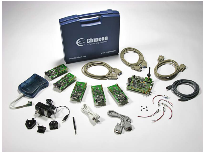
Figure 5.1: CC2420 ZigBee DK Development Kit
