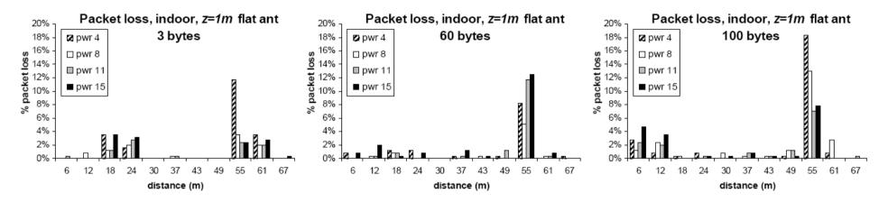
Indoor range test, 1m node height, flat antenna orientation, three packet sizes
