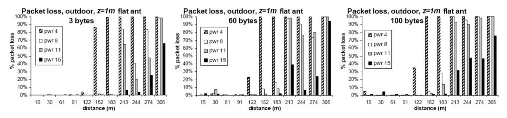
Outdoor range test, 1m node height, flat antenna orientation, three packet sizes
