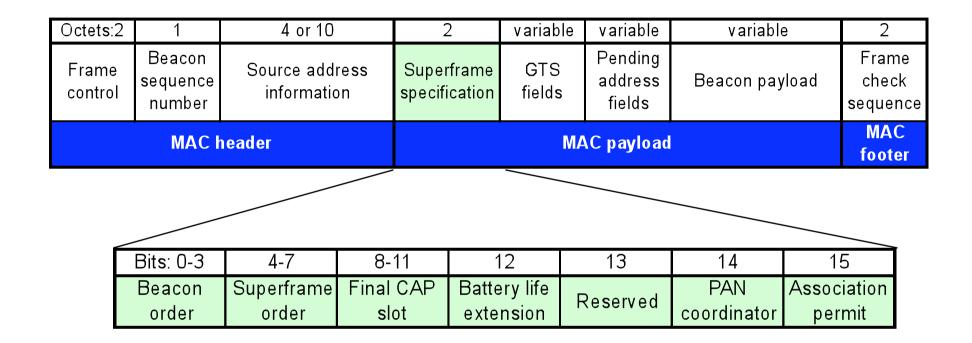
Beacon Order (BO): Describes the interval at which the coordinator shall transmit its beacon frames.
