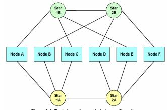
Figure 1-4: Dual channel cascaded star configuration.
