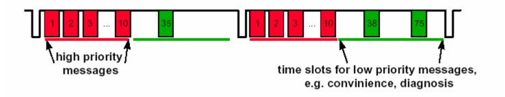
Slots with fixed priorities are reserved for synchronous messages. These slots are assigned in every cycle (1-10) and allow a deterministic analysis of message latencies.
