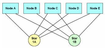
Figure 1-2: Dual channel single star configuration.
