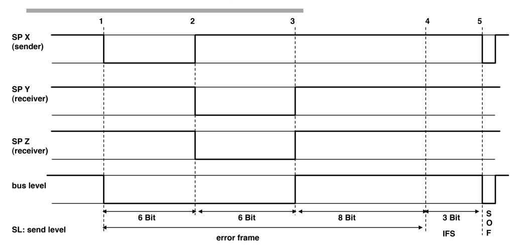
time to re-transmit a faulty message frame: min. error recovery time: 23 bit times
