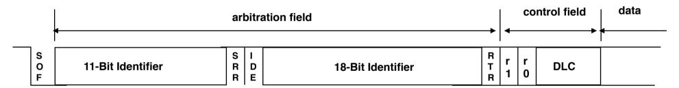
RTR: Remote Transmission Request. In Data Frame: RTR = dominant. In Remote Frame: RTR = recessive.
