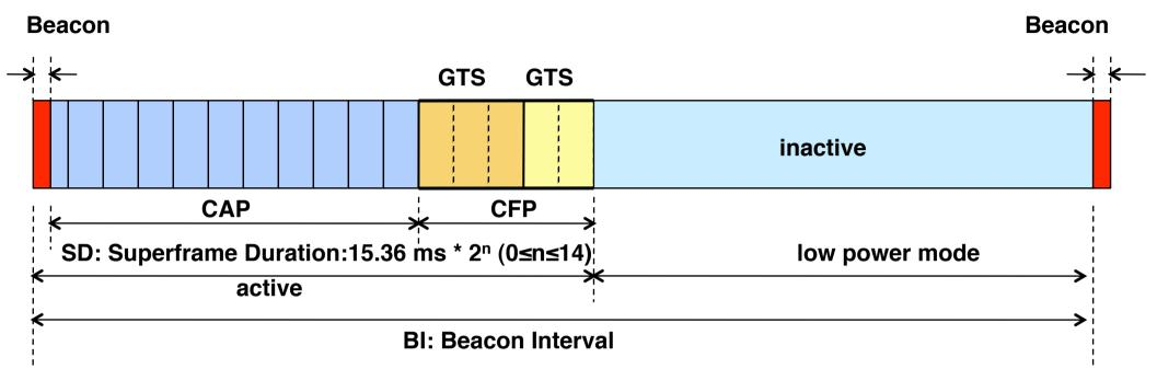
**Beacon:** sent by PAN coordinator in the first slot of the superframe. Contains network information, frame structure and notification of pending node messages.
