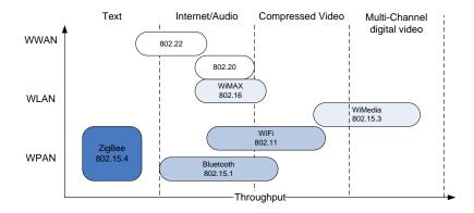
Definition Wireless Sensor/Actuator-Networks Wireless Communication
