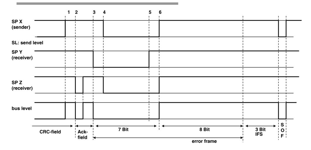
time to re-transmit: min. error recovery time: 20 bit times
