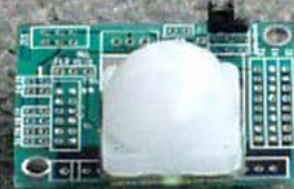
PIR: Passive InfraRed motion detector
