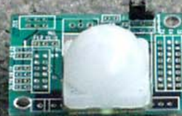
PIR: Passive InfraRed motion detector
