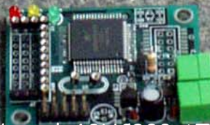
TINY basic board: 68HC908 AZ60: 60 k Flash, 2 k RAM, CAN, serial, extension ports for piggy-back boards.
